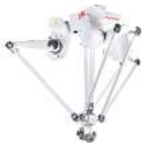
Fig. 13. Robot industrial IRB 390 FlexPacker
